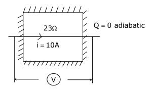
$$W_{electric} = i^2R = (10^2 \times 20) \text{ watts} = -2.3 \text{kw (on system)}$$
