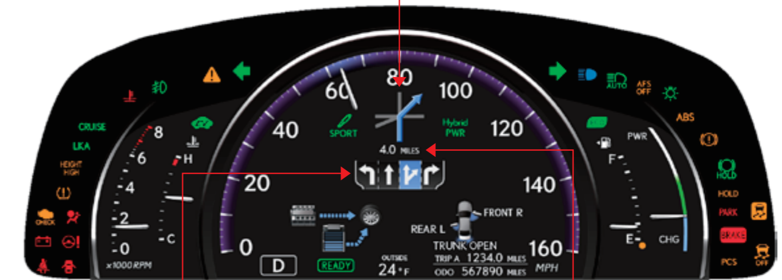
Traffic lane information
