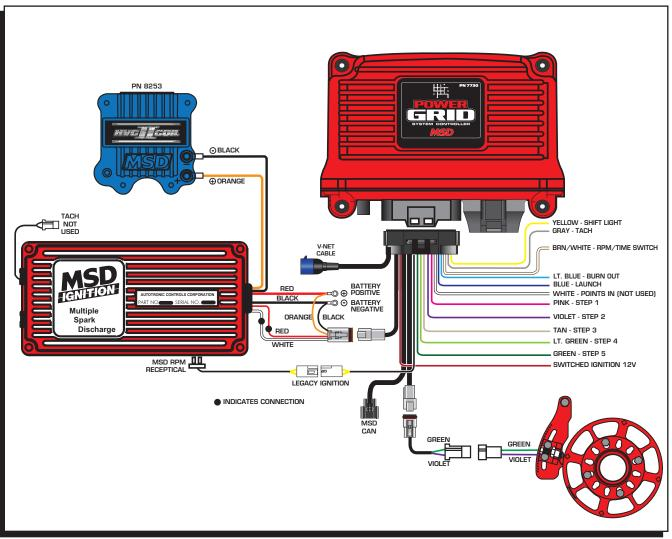
Figure 6 Wiring the Power Grid Controller to MSD 6AL.
