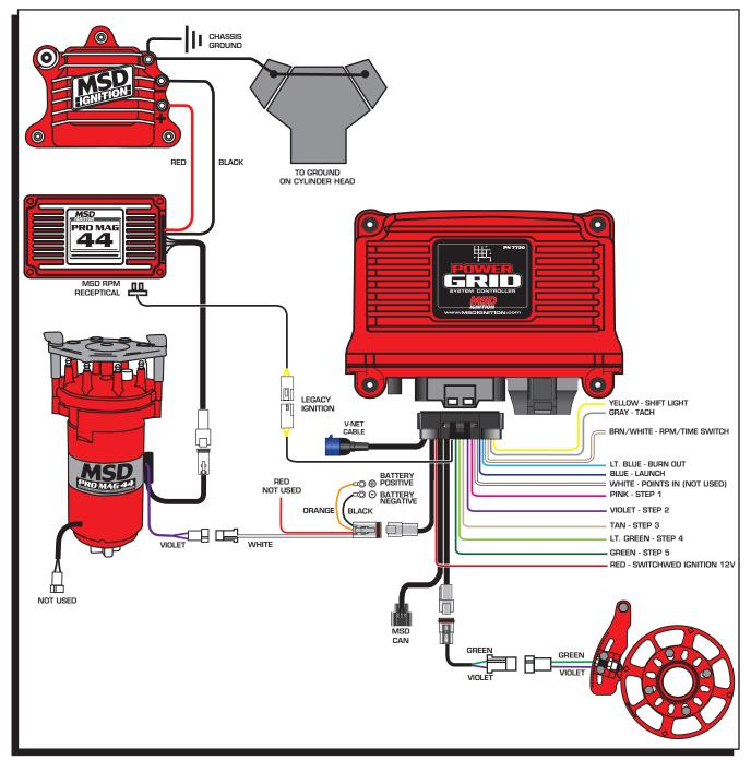
Figure 5 Wiring the Power Grid Controller to Pro-Mag.
