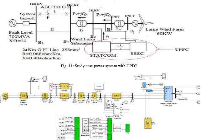
Fig.12 Simulink model of uncompensated system With UPFC
