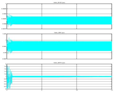
Fig. 4 Effect of change in wind speed on output Voltages at various buses with Resistive load
