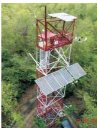
Eddy covariance tower in Haldwani (Uttarakhand) area for measuring CO 2 and water vapour exchange
